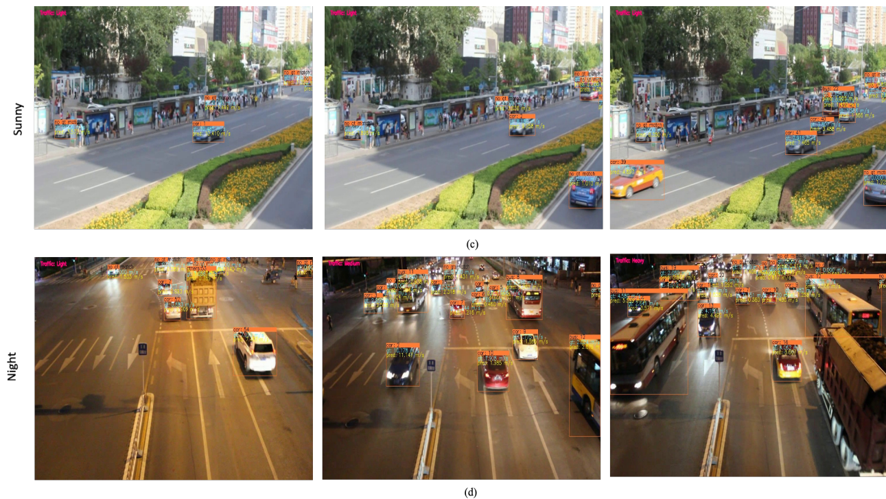
Figure 6: Videos/Images showing speed and traffic density estimation of our method in a) cloudy scene b) rainy scene c) sunny scene d) night scene with light. Full videos here: http://dx.doi.org/10.1117/12.2663643.1 , http://dx.doi.org/10.1117/12.2663643.2 , http://dx.doi.org/10.1117/12.2663643.3 , http://dx.doi.org/10.1117/12.2663643.4
